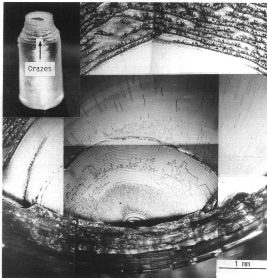
Figure 5 Appearance and fracture surface of the fatigue specimen presoaked in methanol for 24 h. N_f = 3750480
